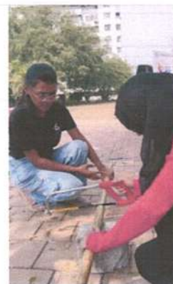
Cutting of Bamboo using a hacksaw
