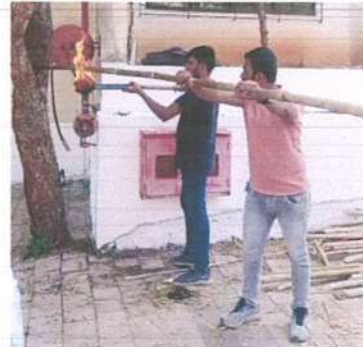
Heating bamboo with Flame torch
